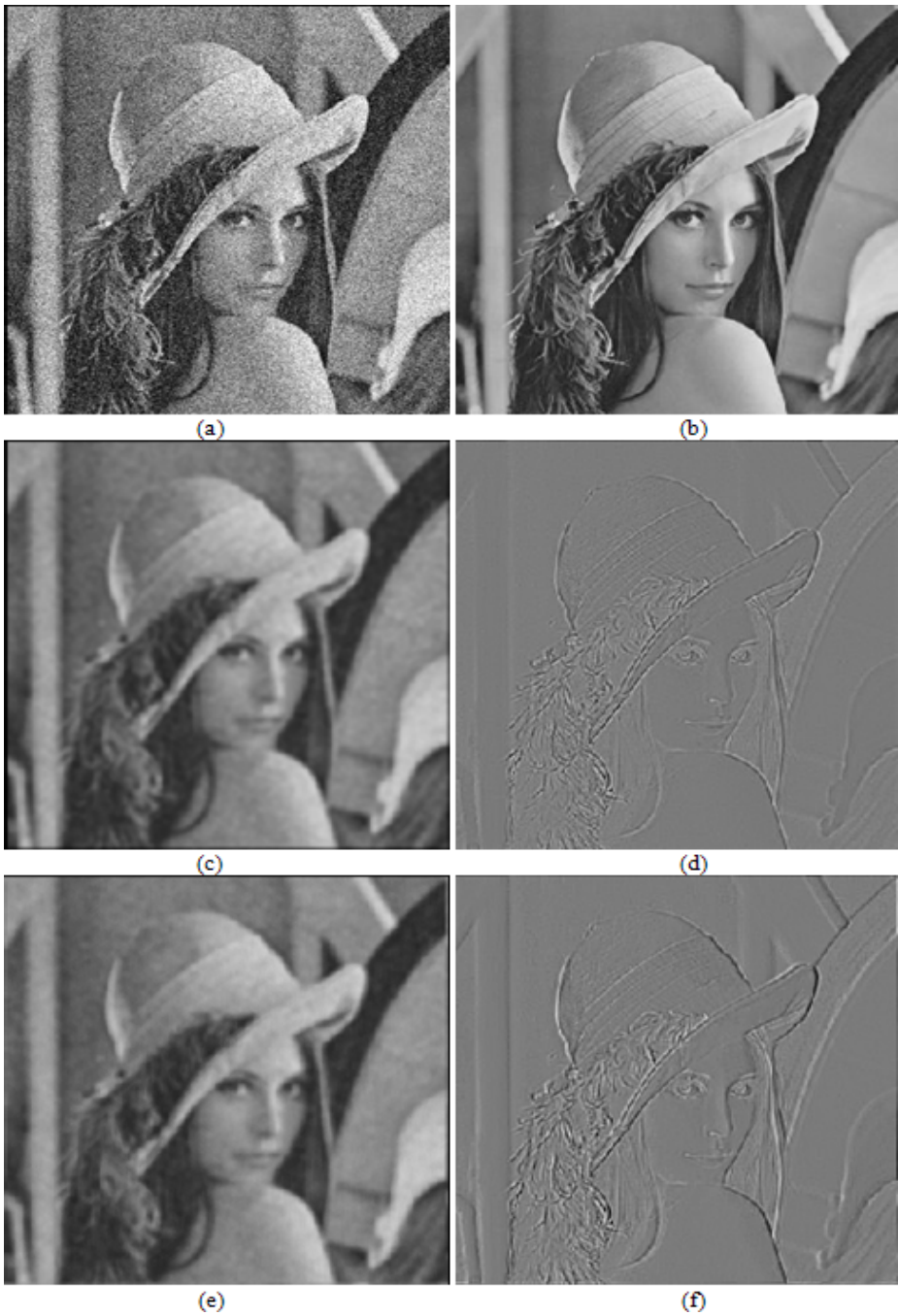
Fig. 6. (a) and (b) are test images for convolution operation with low-pass and high-pass transfer functions, respectively. (c) and (d) are the output images produced by Matlab software. (e) and (f) are the results from hardware simulation.
